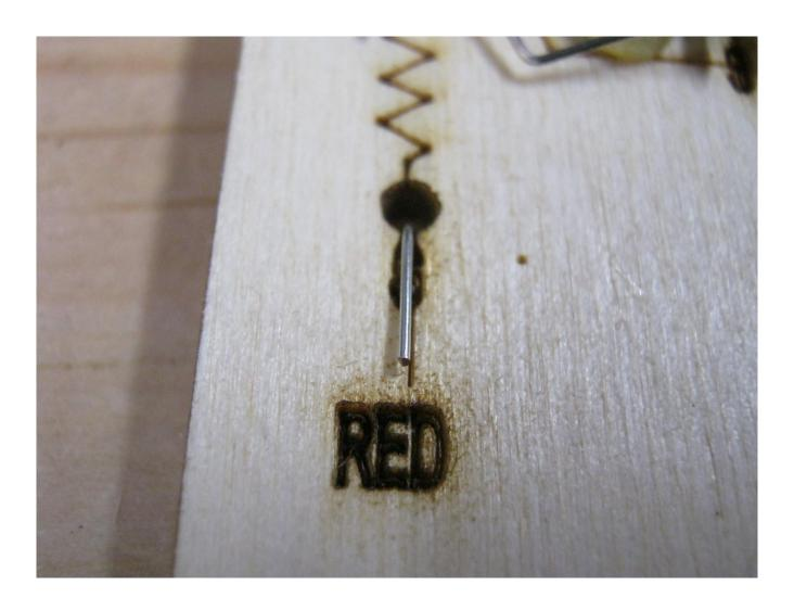
The other resistor lead is bent over towards the RED lettering and cut off as per the woodburned schematic line end.
