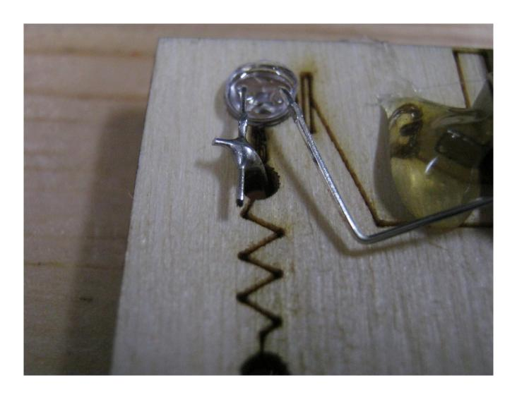
You can bend the resistor lead closest to the LED over the left LED lead, solder the 2 leads together and cut the extra leads off.
