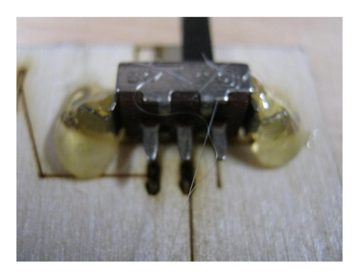
Hot glue the slide switch tabs to the wooden circuit board. Don't use too much glue so the solder tabs remain clear to solder to.
