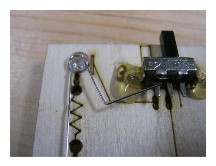
Push the LED through the large LED hole with the flat side of the case (which is also the shorter lead on the LED) oriented to the right...closest to the switch.
