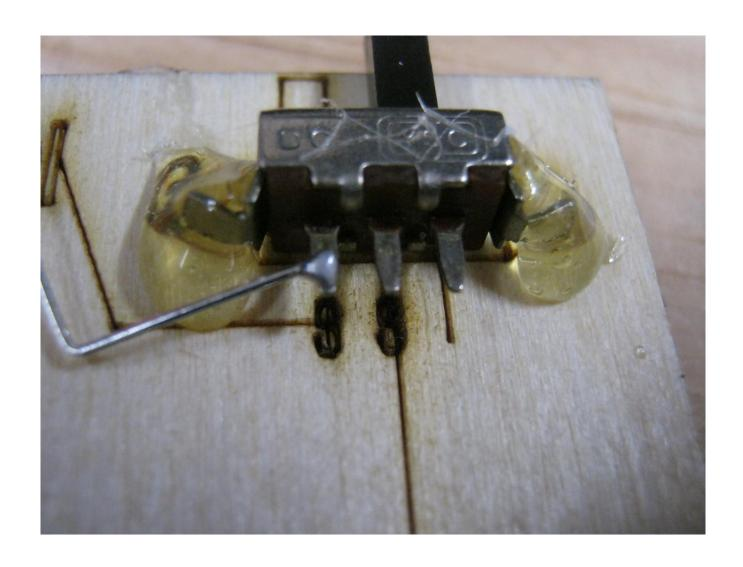
Solder that short lead to the leftmost pin on the switch. Cut off any excess lead if there is any so it doesn't get close to the middle pin on the switch.
