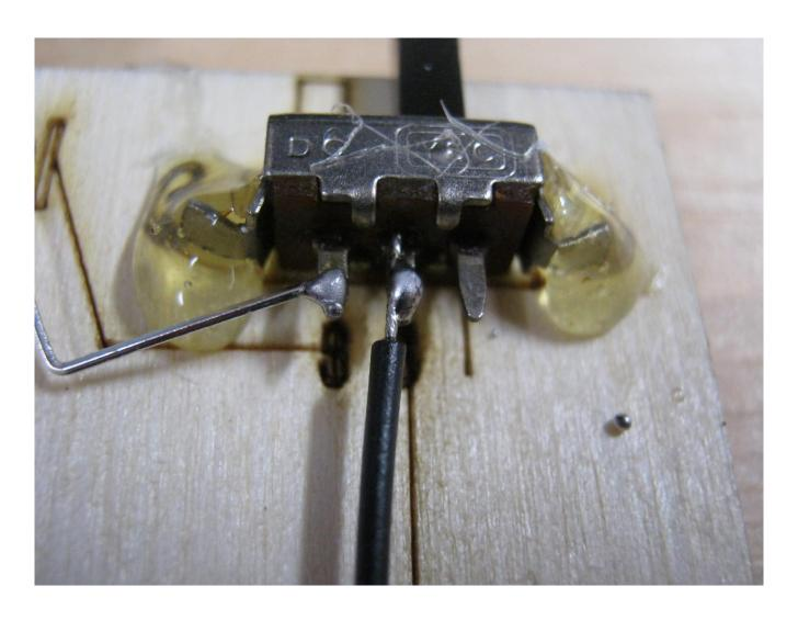
Solder the 9 volt battery snap wire to the center pin of the slide switch...
