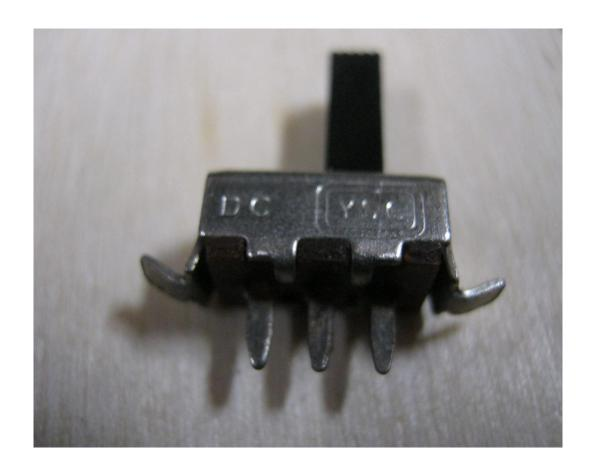
Bend up the outside case tabs of the slide switch using a small pair of needle nose pliers....
