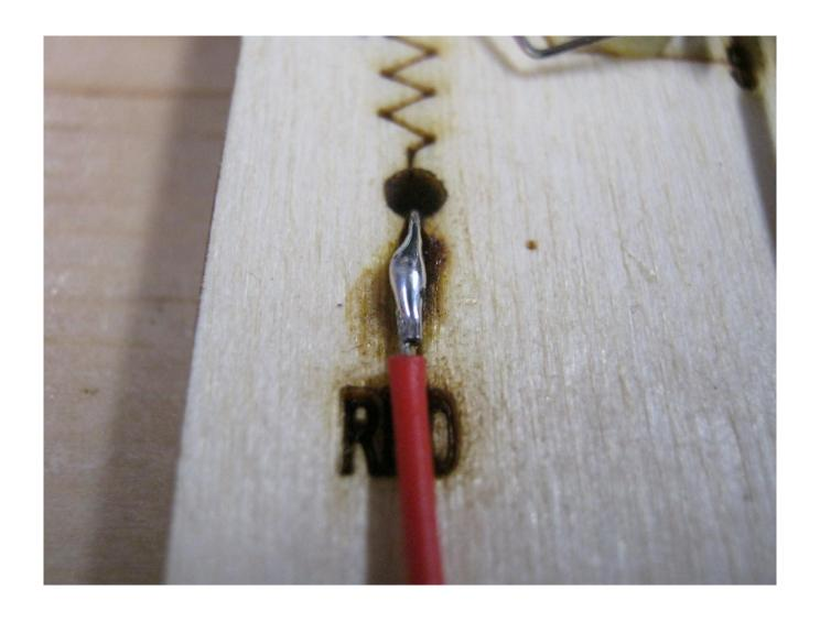
Solder the resistor lead and RED 9 volt battery snap wire together...
